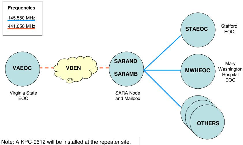
Note: A KPC-9612 will be installed at the repeater site, which will allow us to cross band to UHF packet and connect to VDEN (Virginia Digital Emergency Network) and the Virginia EOC.
