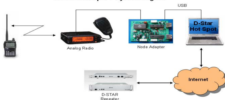
D-STAR Hot Spot - System Diagram
